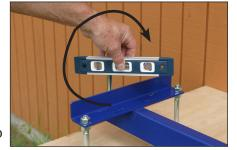
CHECKING THE PITCH CHECK FOR LEVEL
