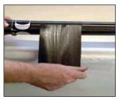
9. Apply the shrinktape over the patch. Start the shrinktape on the unsanded area of the shaft one inch from the repair area. The tape should advance about 1/8 - 1/4 of an inch with each shaft revolution. In this way, the tape will wrap onto itself and result in four layers of tape over the patch. The tape should extend 1" on either side of the repair. This operation works best with v-blocks on a table.
